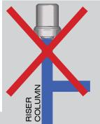
In locating the water hammer correct position in a system, it is important to avoid creating areas where stagnant water may remain, i.e. situations where bacterial colonies can proliferate. For instance, installations at the top of a riser column can create areas with still water ("dead zones"), even though the water hammer arrester will function properly. Consequently, this kind of installation must be avoided.
