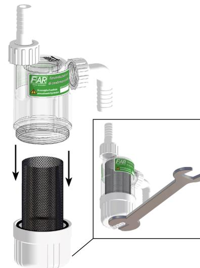
**1** Unscrew the lower part of the neutralizer. On the lower part there is a support for a 13mm wrench to facilitate the opening.
