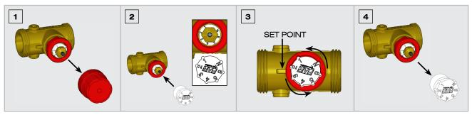
Completely unscrew the handle by turning it anticlockwise.
